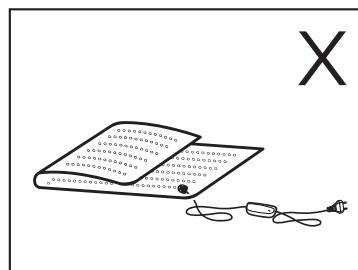
Do not use the blanket where the blanket or the power cord are easily trapped or folded, e.g., on an adjustable bed, a sofa-bed, or an office chair with wheels.
