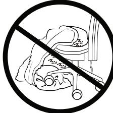
The electronic components inside the controller may cause the controller slightly warm when the electric blanket is in use. Therefore, the controller must not be covered or placed on top of any heating sources when it is in operation.
